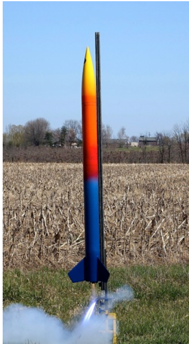
Finally, Pat Ralph once again flew his original LOC/Precision Magnum (left) which was set-up for dual deployment and flown on a CTI J449 Bluestreak motor to an altitude of 2885 feet (right).
