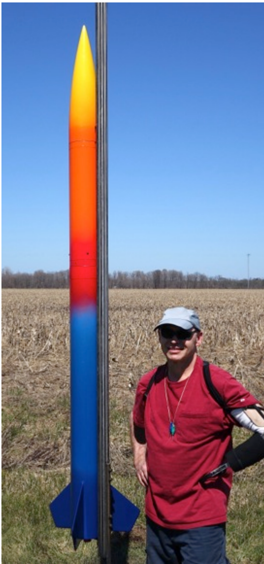
Finally, Pat Ralph once again flew his original LOC/Precision Magnum (left) which was set-up for dual deployment and flown on a CTI J449 Bluestreak motor to an altitude of 2885 feet (right).
