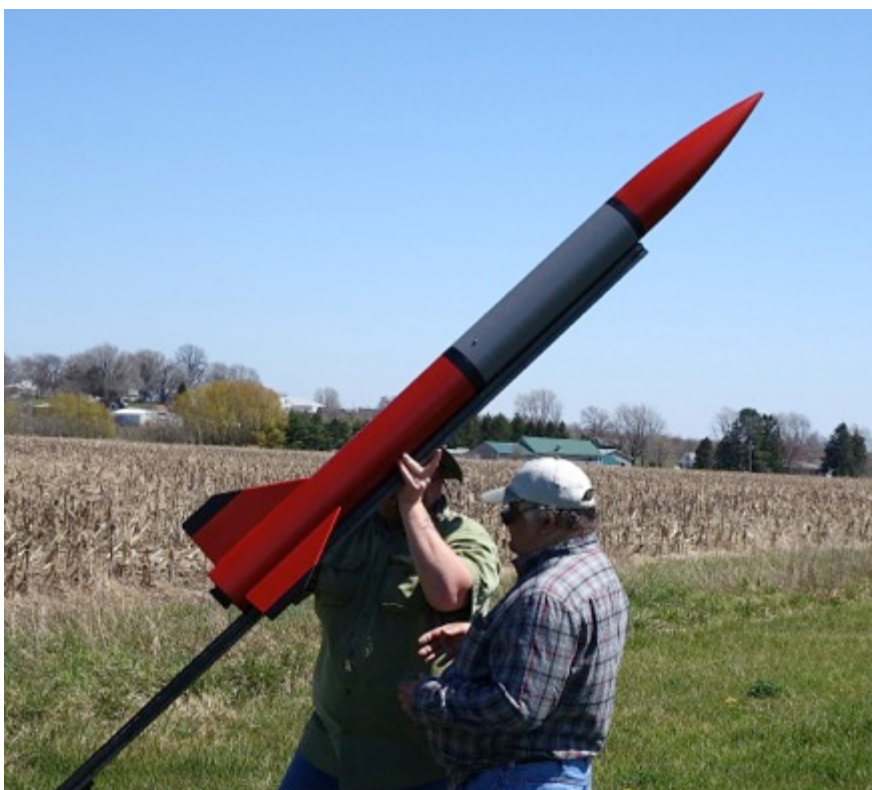
Andrew Kleinhenz and Bruce Levinson (below) load the Super Saffron up for a second flight with a Research J480, which flew to 2105 feet (right).
