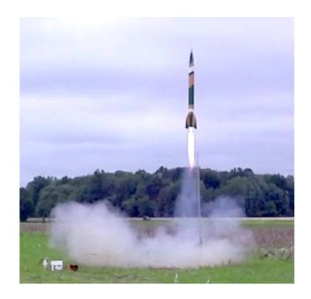
Mike Momenee (left) was finally able to make it to one of our launches and brought his scratch built 6" V-2 which he flew with an AT K1000 motor to an altitude of 2622 feet (above).
