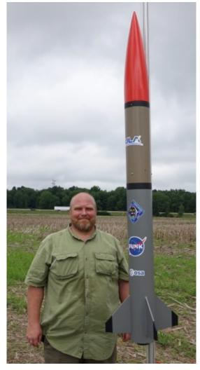
Andrew Kleinhenz (left) flew his 5.5" diameter, 6 foot tall rocket called "Earth, Wind and Fire" hence the "Funk" sticker on it. It flew on a Research 54mm three grain RCS Purple for a perfect flight to 2970 feet. Then another flight on a 54mm 3 grain NASSA K2 Fast which weathercocked badly and nearly landed on the turnpike.
