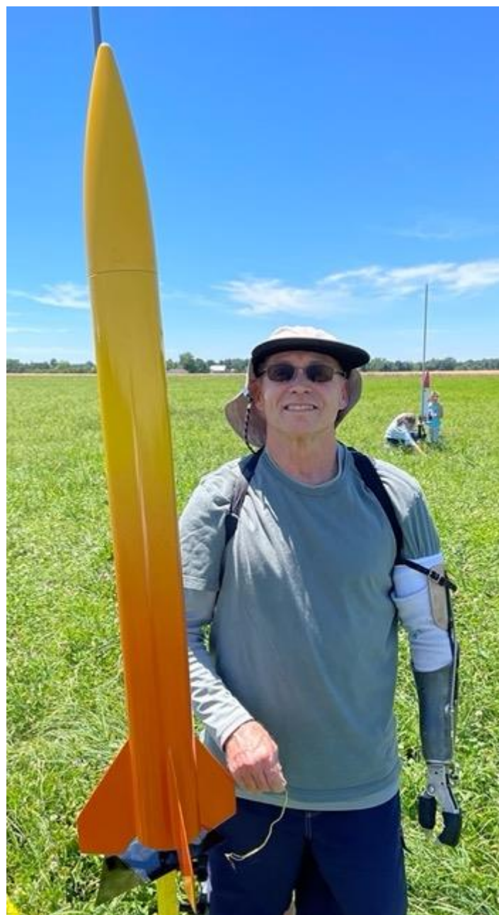
Pat Ralph (right) puts his LOC/Precision "LOC 4" on the pad. The CTI H64 motor took the rocket to an altitude of 1700 feet.
