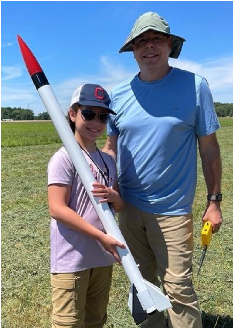
Pete Taran and Evangeline ready to take their LOC/Precision "Tomahawk" out to the pad. It was equipped with dual-deploy and a GPS tracker. It flew to 3500 feet with a CTI H250 Green motor.
