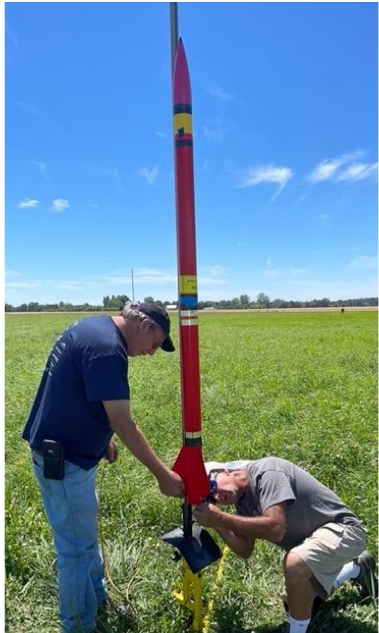
Mark Coburn (kneeling) hooking up the igniter on his rocket named (wait for it!) “Bug Juice” which he flew with a 54mm Research J460 motor to an altitude of 4800 feet. Steve Eves assisted.
