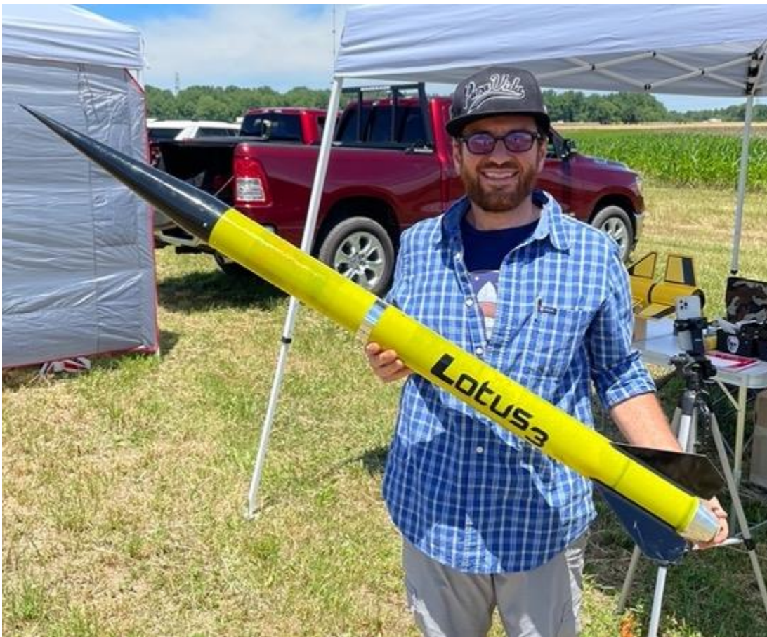
Casey Anderson (Left) with his "Lotus 3" which featured a clear yellow fiberglass airframe (cool!). He flew it to an altitude of 1050 feet on a CTI H220 motor.
