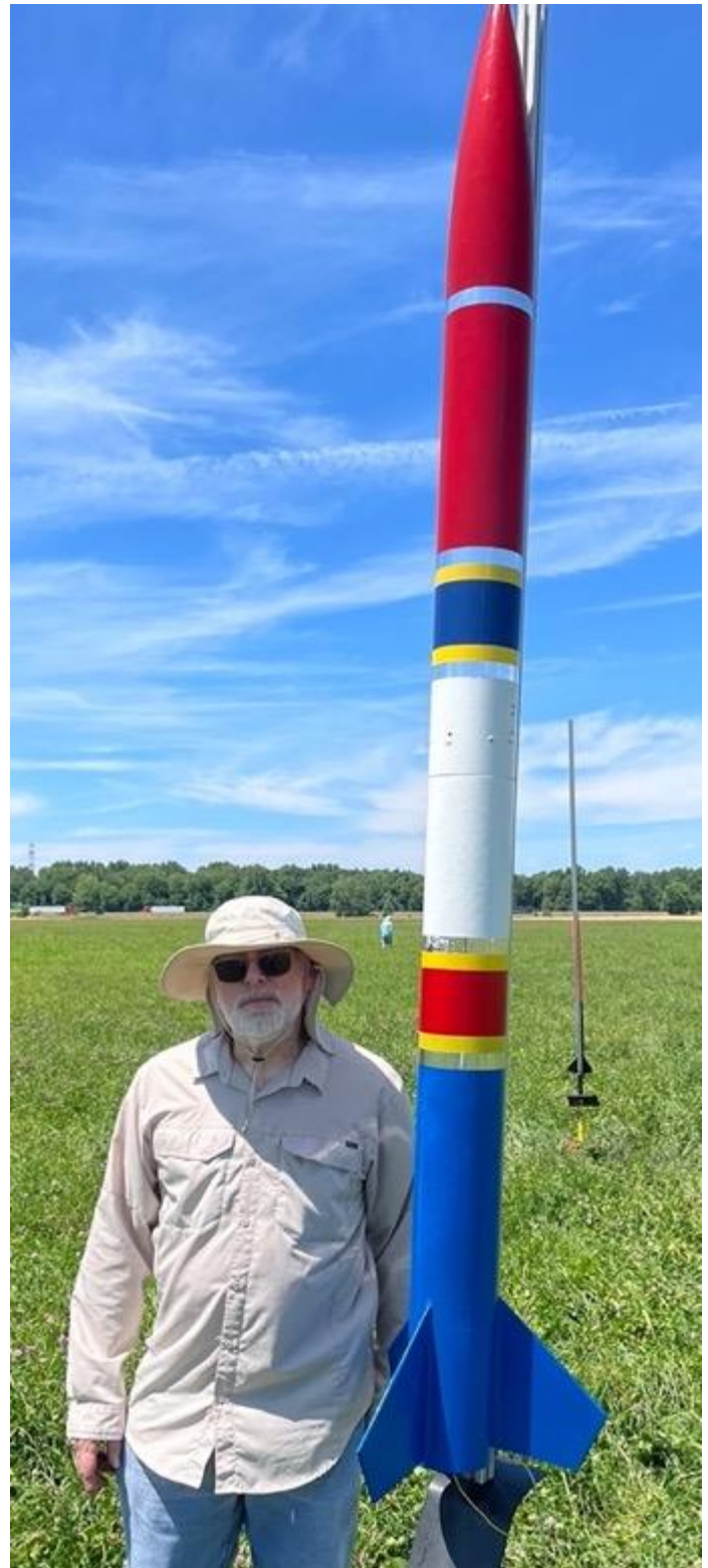
Pete and Evangeline Taran (above) flew her LOC/Precision 4" "Goblin" with an AT I327 Dark Matter motor to an altitude of 3500 feet. An original Estes "Goblin" is held next to it for a size comparison.
