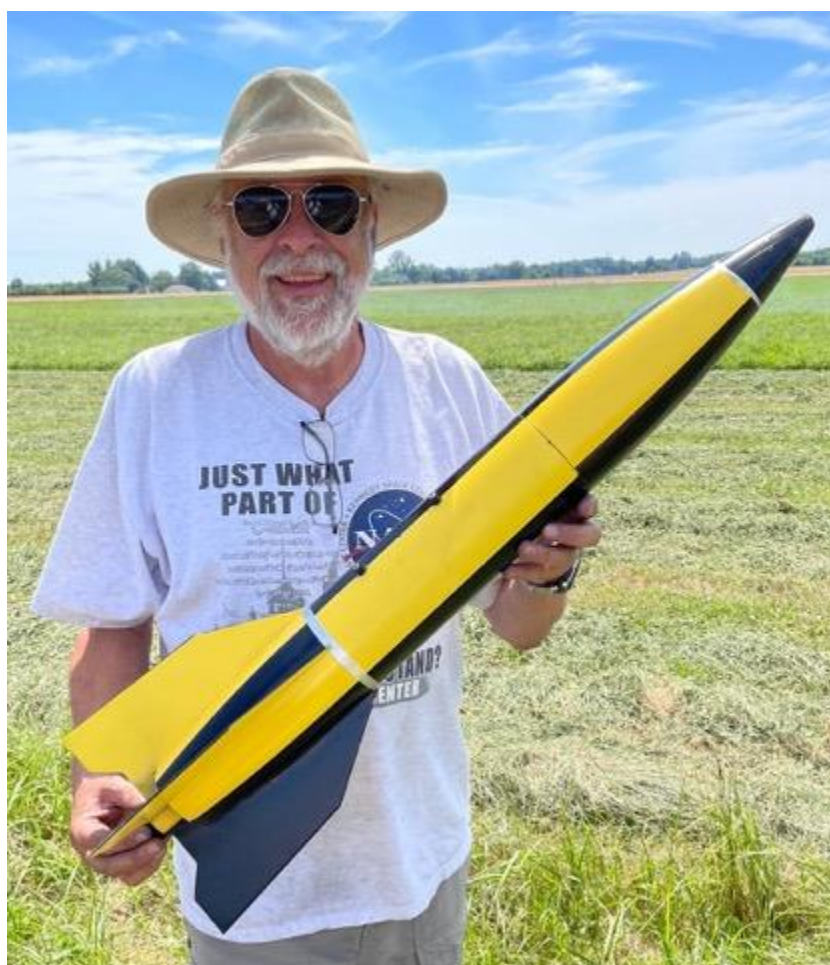
Mark Hanna (right) heading out to the pads with his 4" LOC/Precision V-2 that he flew to an altitude of 1100 feet with a CTI H133 motor.
