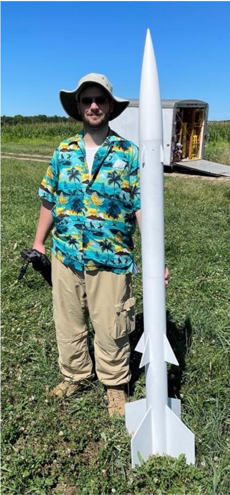
Chris Feyerchak flew his LOC/Precision "Nike-Zeus" with an electronics bay modification on an AT H180 W motor for a Level 1 certification flight to an altitude of only 632 feet! But he got the certification! Chris' flight was one of four L1 certification flights done at the launch.
