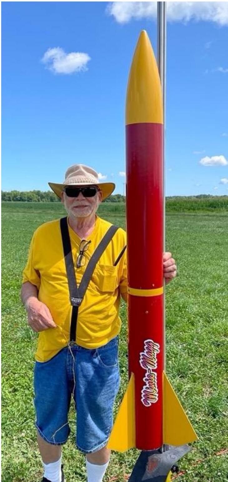
Terry Habegger (left) puts his extended LOC/Precision “Mini-Magg” which he calls his “LOC Red Rocket” on the pad. He flew it with an AT J420 R motor and was expecting an altitude of 3000 feet, but the electronics didn’t deploy the recovery system.
