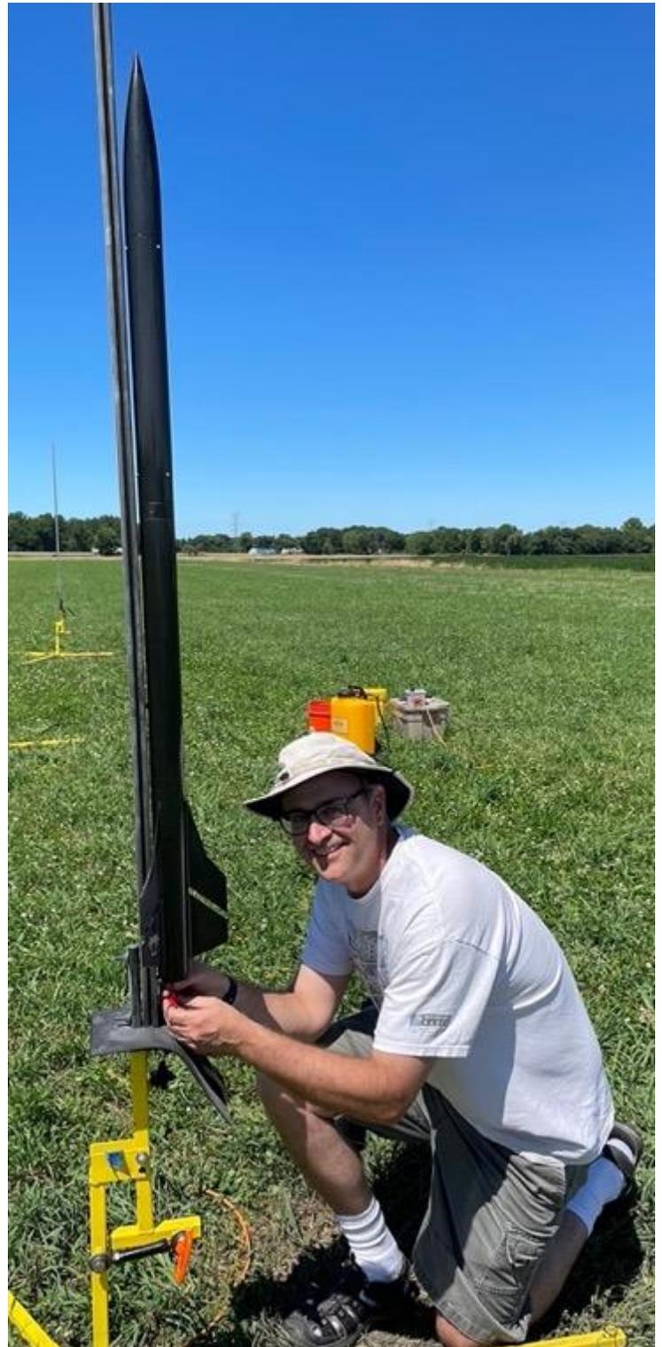
Andy Brown (left) hooks up the igniter on his Mach 1 "Viper" which he flew with an AT H180 motor to an altitude of 2200 feet. He also flew an "Alien Interceptor" with an AT H128 motor.
