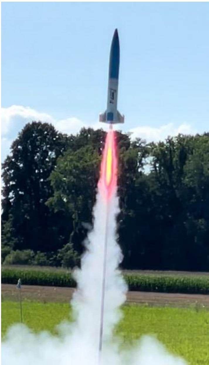
Pete Taran's 4" LOC/Precision "T-LOC" takes to the air with an AT H268 R motor which took it to an altitude of 3000 feet (left).
