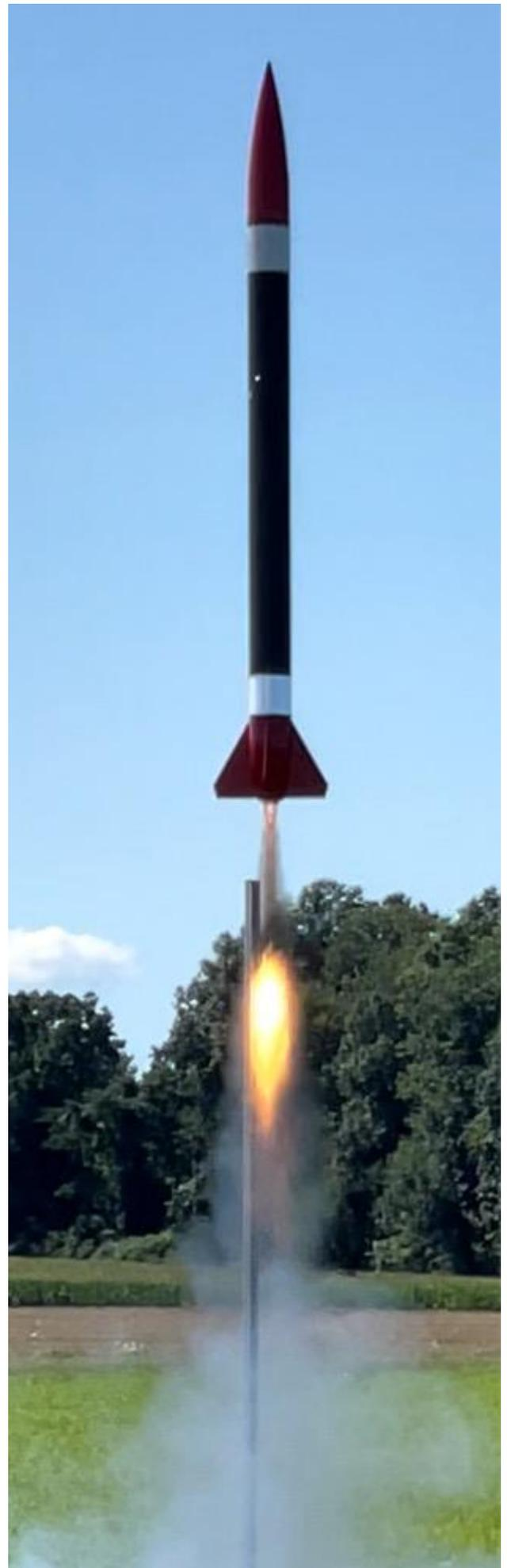
Steve Eves (above) with another of original LOC/Precision rockets from the 80's, a "Syonic" which he flew with a Research K600 motor to an altitude of 3000 feet using NASSA K2 Fast Propellant.
