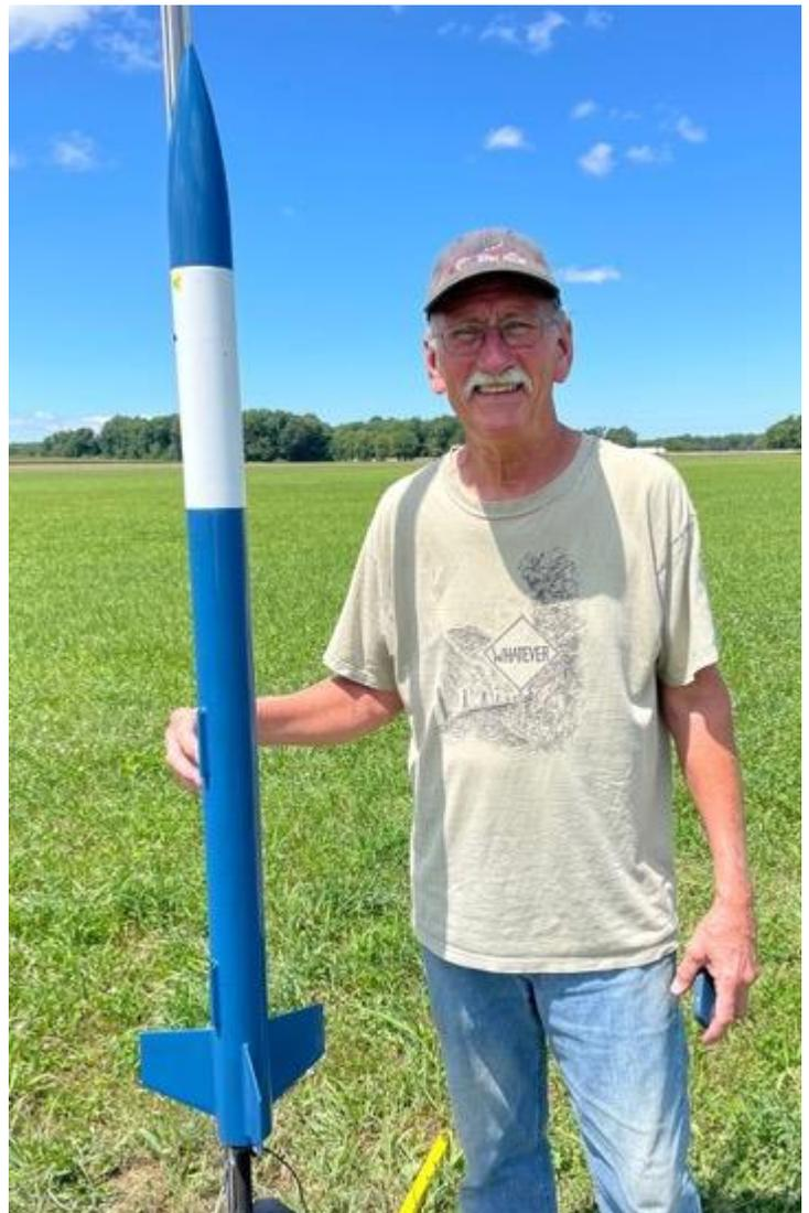
Mark Flickenscher (right) puts his scratch-built "Blue Streaker" on the pad. He flew it to an altitude of 1800 feet on an AT G64 motor.
