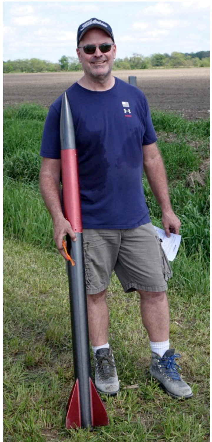
Dave Sears (right) flew his "Caliber ISP" with a Research 54mm I200 White motor to an altitude of 2365 feet.
