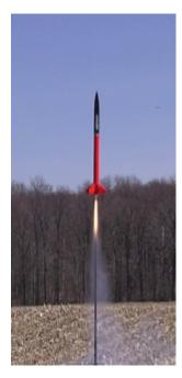
Chris Pearson flew his 4" Katana EX signed by Burt Rutan once again on a Research 54mm K350 using NASSA K2 Slow propellant (left). The almost four second burn and weather cocking took the rocket to over 3000 feet and well into the next field past the tree line which made for the longest walk to recover a rocket at the launch.
