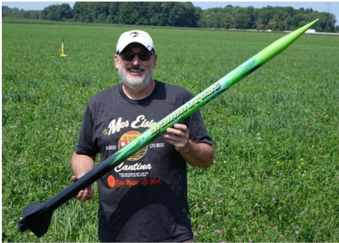
John Bryan on his way to the pads with his Estes "Mammoth" which he flew with an AT E30 motor to an expected altitude of 800 feet.
