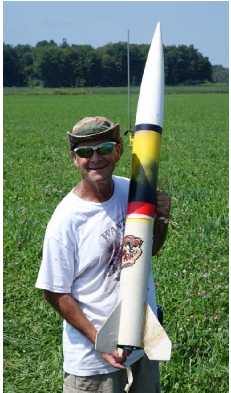
Mark Coburn with his scratch-built "Taz" rocket that he flew with an AT H238 motor.
