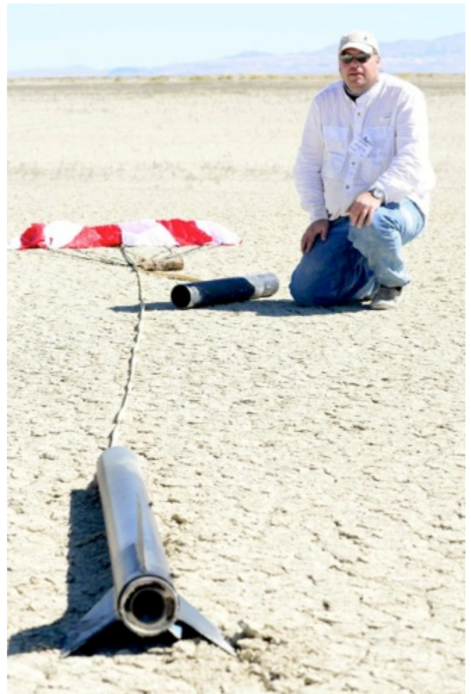
Eric Smedstad (left) with his two-stage rocket on the pad. First stage (right) was recovered perfectly. The second stage lost 2 of its 3 fins but still made it to 80,000 ft.!
