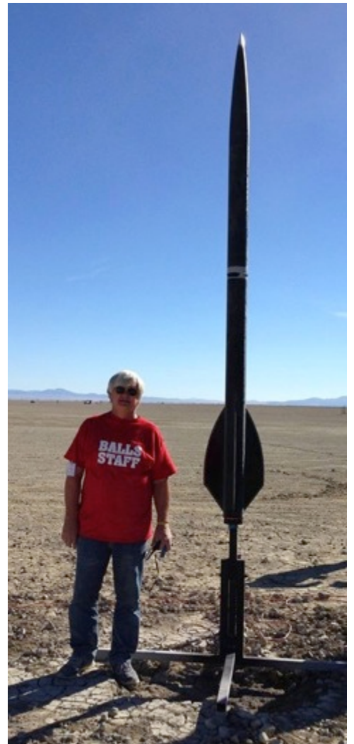
Joe Grubb and "Shape Shifter" (right). This flight went 600 mph to 9300 ft. on an Aerotech M1550R. Recovered 600 yards away with no damage.
