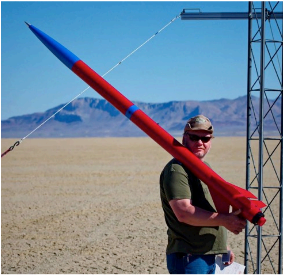
(Left) Neil Anderson with his L3 certification attempt rocket, a minimum diameter with a 98mm Aerotech motor.
