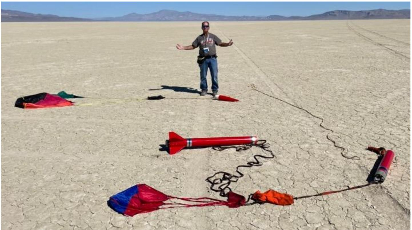
Mark recovers his “Arcas” after the second successful flight on a Research 75mm L1175 using NASSA K2 Fast propellant. The rocket flew to 9500 feet and was recovered undamaged. About the only way to lose your rocket at Balls is if the recovery system fails and it lawn darts into the playa. They can go pretty deep depending on impact velocity and many are unrecoverable.
