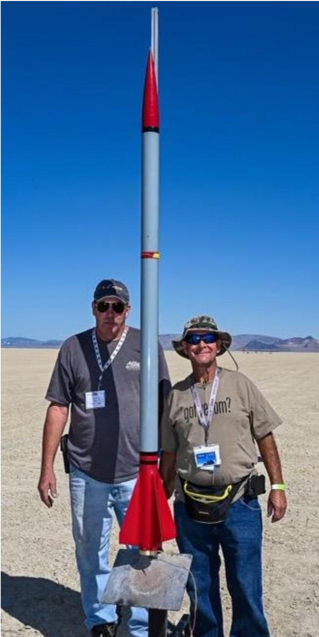
Steve and Mark pose with Steve's "Starchaser" a 3" minimum diameter rocket being flown with Steve's first Research moon-burning motor which simmed out to a L400. It took the rocket to an altitude of 12,300 feet and landed for a perfect recovery.
