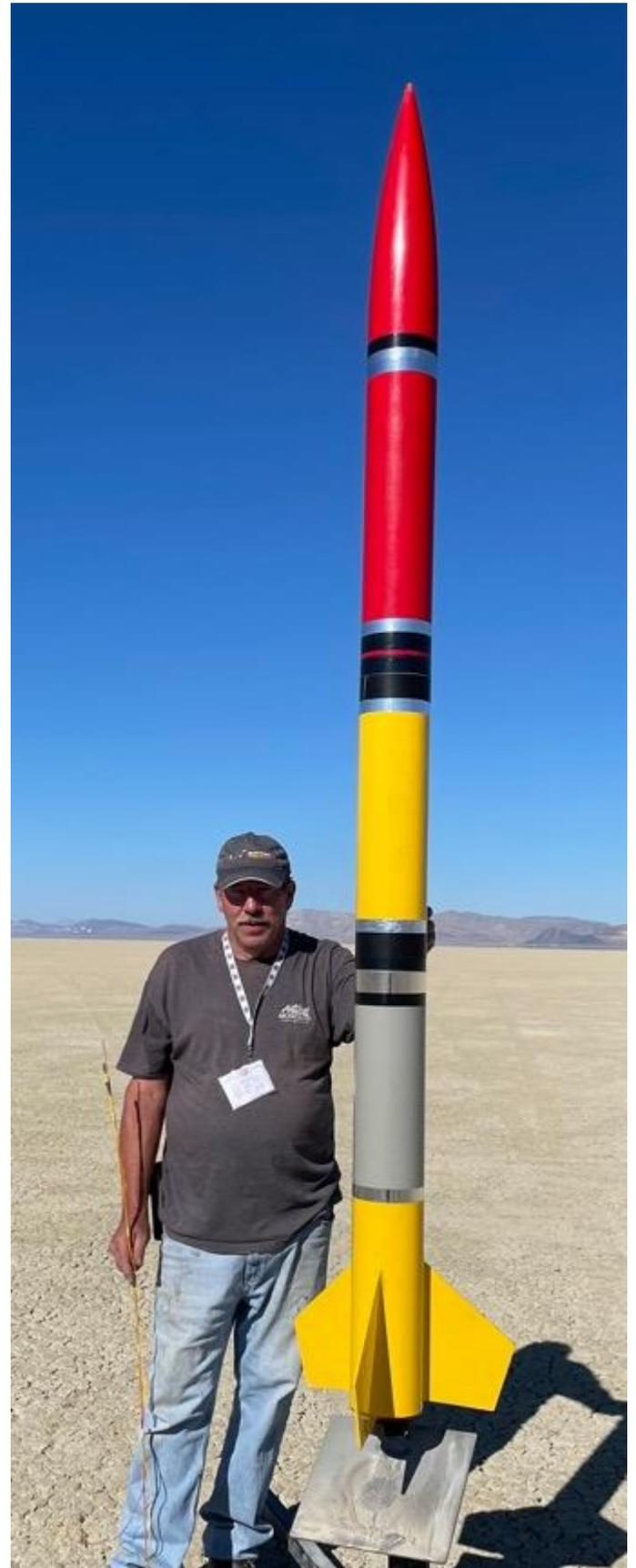
Steve (right) poses with Mark's LOC/Precision "Magnum" ready for its second flight on a Research 75mm M3200 motor using NASSA K2 Fast again. It hit 9,800 feet and had a perfect recovery.
