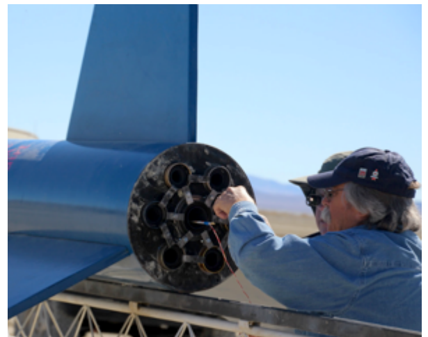
The “Gila Monster” being prepared for flight with insertion of the traditional Balls keg of beer (left). The motors are prepped for flight. One 4” motor and six 3” motors (below).
