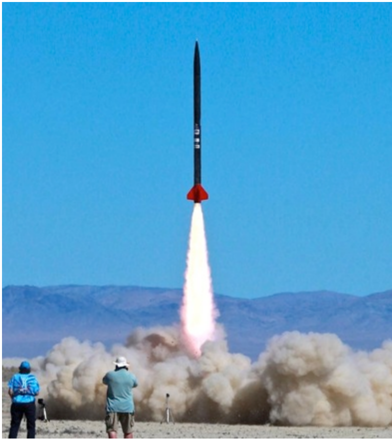
The Rockets magazine “Black Sheep” project rocket takes off under the thrust of a Research P10000 motor (above). The “Black Sheep” in flight (right) which deployed its main parachute at the 40,000 ft. apogee and floated off to the wilderness of Black Rock,
