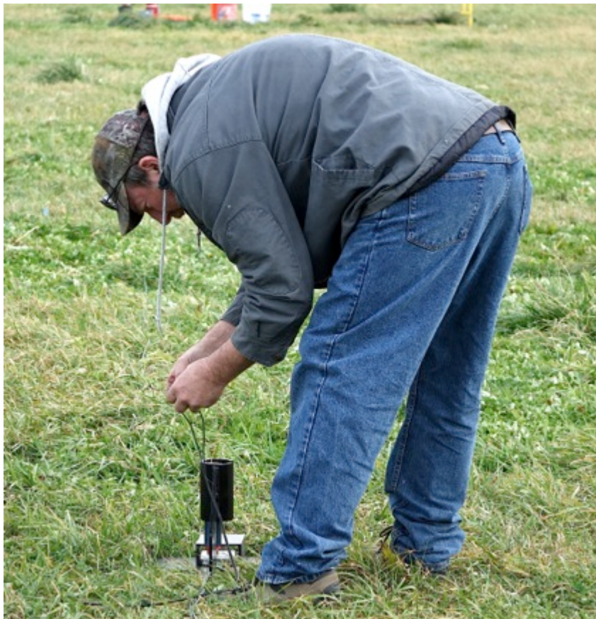
Steve Eves (above) hooking up the ignition leads to a 38mm motor about to be static tested. NOTRA owns a load cell and a Data Logger USB, a computerized motor testing hardware and software system made by Dave Cooper, a NOTRA member.
