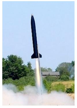
Pat Ralph's only flight was the Super Warlock (left), actually an extended stock LOC/Precision Warlock set up for dual deploy. Flying with a CTI K590 DualThrust motor to 3482 feet with a pretty steep launcher angle because of the stiff winds. The mains fired at 900 feet and it landed right at the perimeter of the field.
