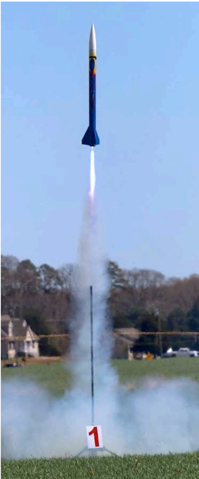
Eric Fadely's "Slap'n the Pig" (above left) flying a 54mm Research K1065 using Terry McCreary's Blue Blazes IV propellant. Someone finally got a pic of Chris Pearson's "Big Six Inch" (above right) flying with a 76mm Research L1500 using NASSA K2 Fast propellant. The rocket reached an altitude of 6700 feet.
