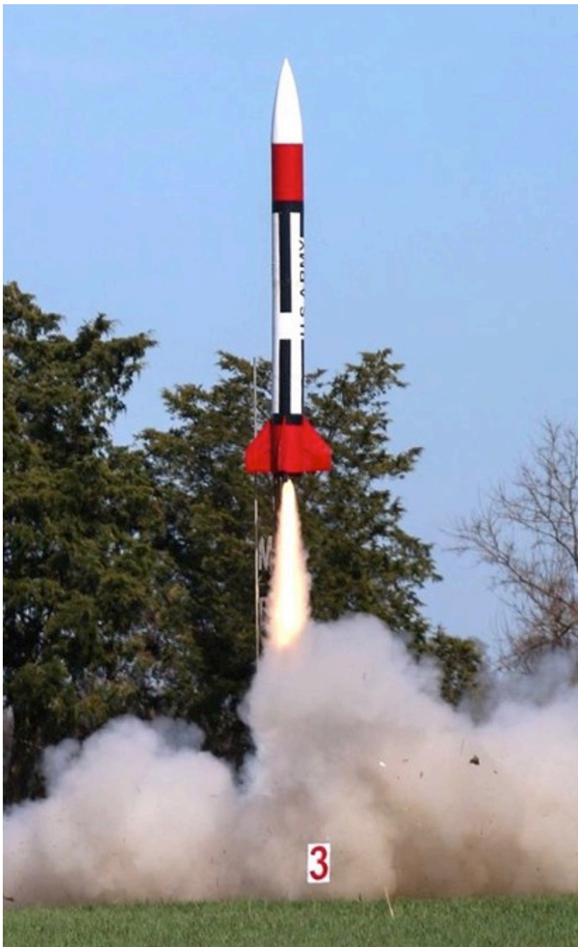
Tom Cohen & Robert DeHate's Full Scale Patriot (above left) weighing in at 210 lbs, flew on a CTI N5600 to about 1,700'. She stands 19' tall, 16" in diameter and is made from composite carbon fiber and fiberglass materials.
