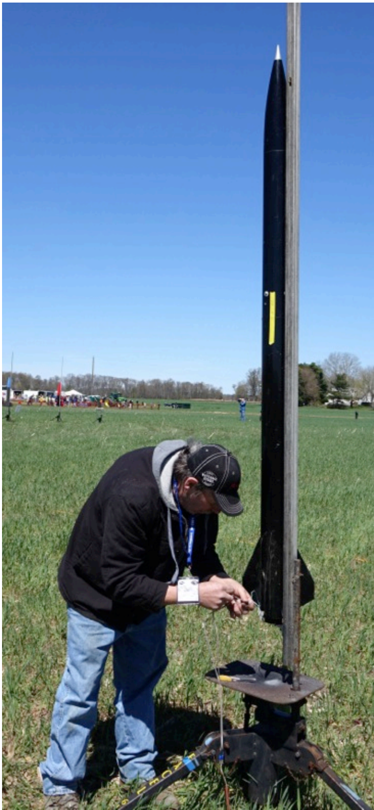
Steve Eves (above left) installing the igniter in his 4" black "Mad Dog" which flew on a Research J480 to 2300 feet only to be drug through the irrigation ditch by the chute and covered with mud. Chris Pearson (above right) with his prototype LOC/Precision "Galactic Explorer" with a Research K615 "Mid-Range Red" motor to an altitude of 3400 feet with perfect dual-deploy recovery.
