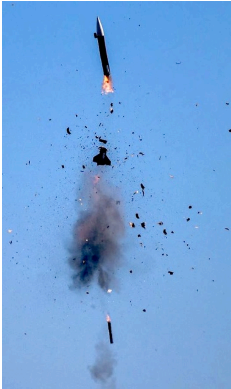
Mike Showalter's 2/3 Scale Patriot (above left) stands 10.5' tall, 9.5" in diameter and weighs 89 lbs on the pad. It was launched on a Research 115mm N3100 motor and the altitude was expected to be 8,500'. Unfortunately the motor cato'ed in mid-burn (above right), blowing the rocket in half.
