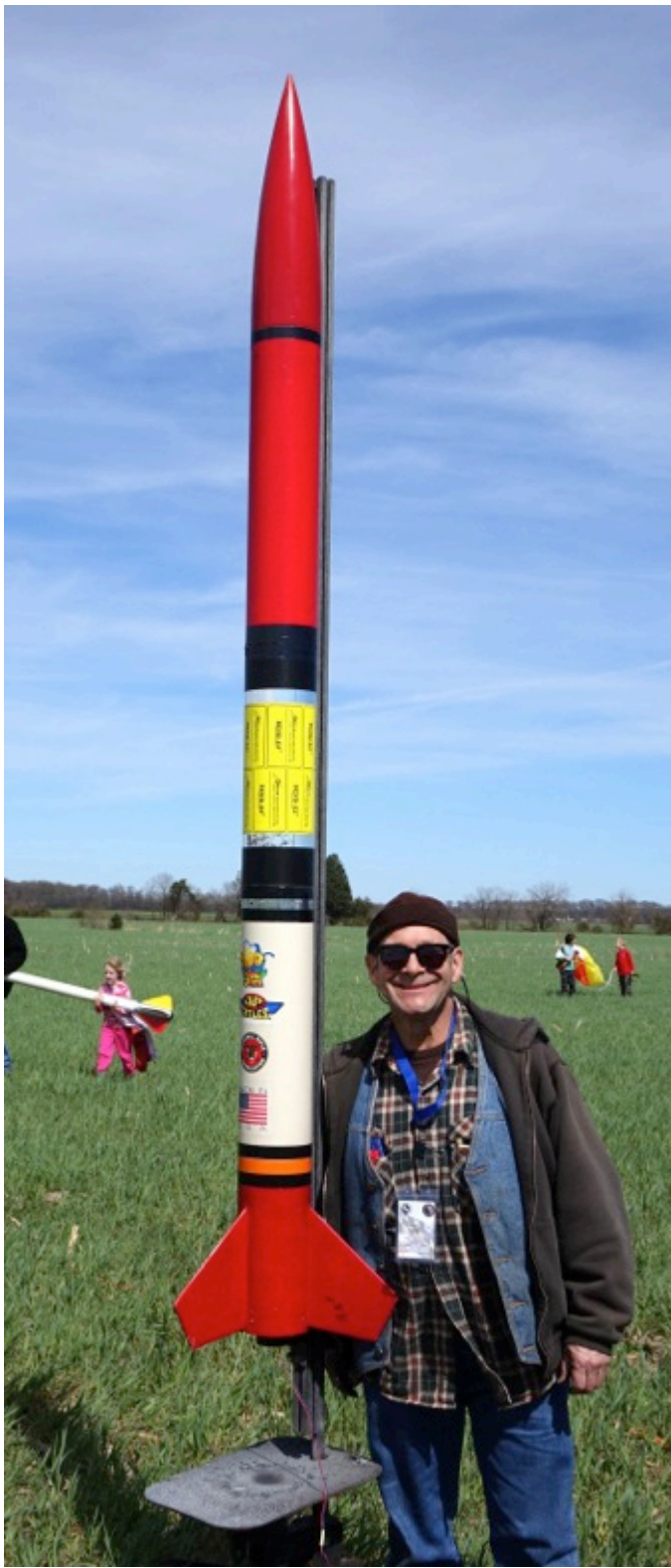
Mark Coburn with his LOC/Precision "Bug Juice" on the pad (above left). The Bug Juice in flight (above right) with a 54mm Research K235 motor using NASSA K2 Slow propellant, which took the rocket to 3120 feet.
