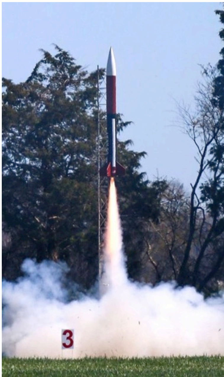
Mike Showalter's 2/3 Scale Patriot (above left) stands 10.5' tall, 9.5" in diameter and weighs 89 lbs on the pad. It was launched on a Research 115mm N3100 motor and the altitude was expected to be 8,500'. Unfortunately the motor cato'ed in mid-burn (above right), blowing the rocket in half.
