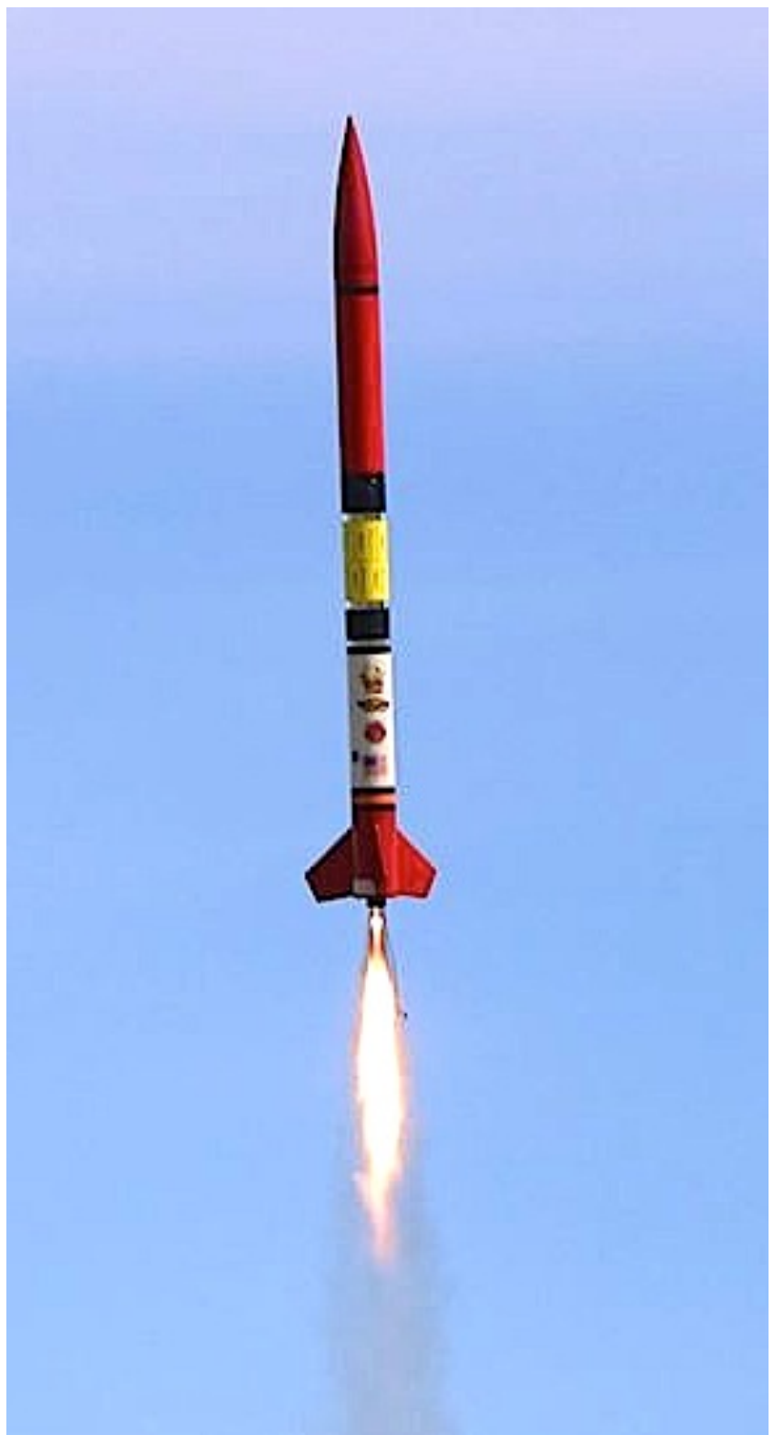
Mark Coburn with his LOC/Precision "Bug Juice" on the pad (above left). The Bug Juice in flight (above right) with a 54mm Research K235 motor using NASSA K2 Slow propellant, which took the rocket to 3120 feet.
