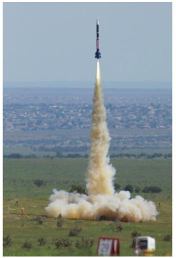
The first rocket that was flown, shown at left, was called the "Stars 'N' Stripes Rocket" and painted in red, white and blue. It was 20 feet tall and powered by an O motor (manufacturer unknown) but must have been really heavy since its predicted altitude was only 5000 feet! It was carrying several active payloads, which it deployed upon descent.
