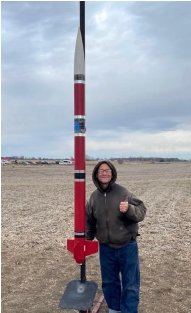
Mark Coburn with his extended LOC/Precision "EZI-65" which he flew with an AT K550W motor.
