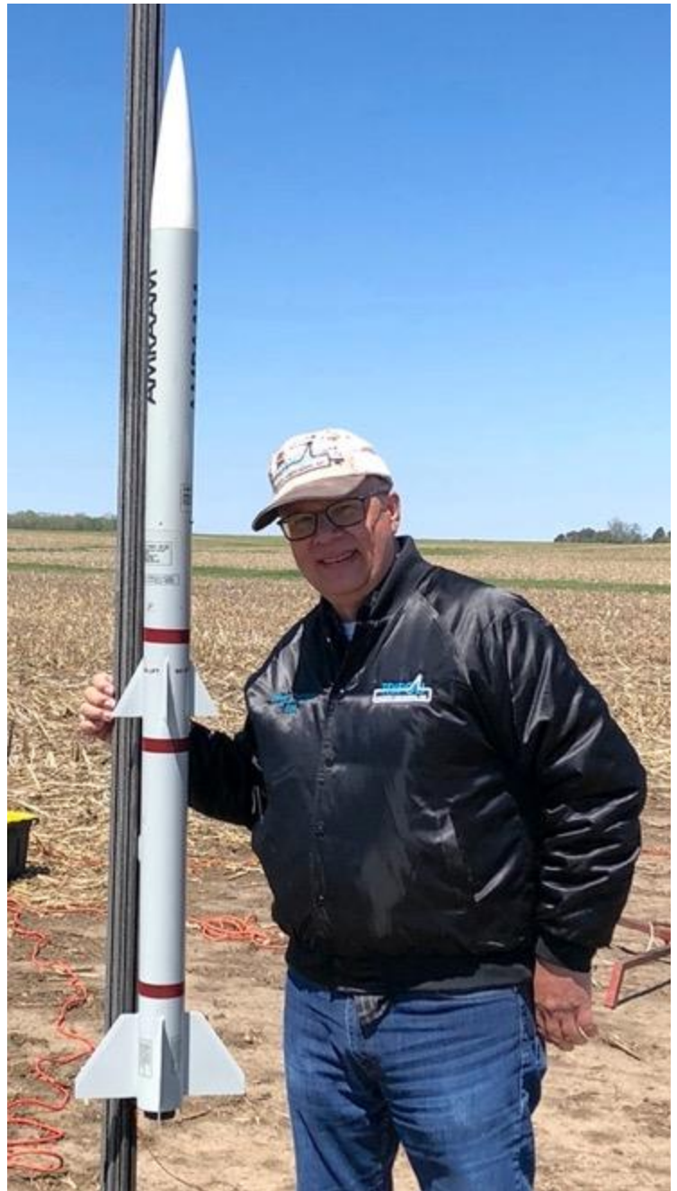
Chris Pearson (right) flew his 3" PML AMRAAM on a CTI I205 IMax to 1900 feet, much better than the paltry 1100 feet he achieved on a H motor at the last launch. Recovery was by Jolly Logic Chute Release.
