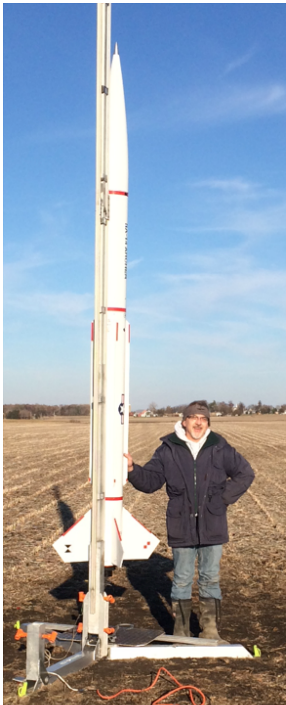
Jim Siebyl (above) poses with his 7.5" "Ultra Archer" prior to its flight with an AT M4500 Super Thunder motor, which took it to 5600 feet in a straight up flight. At right is a long-shot pic of the take-off.
