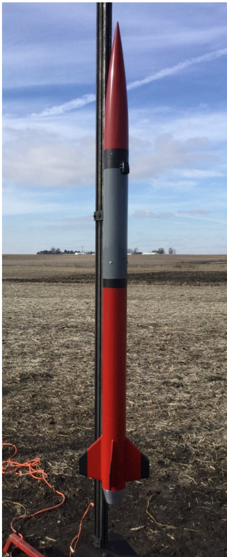
Andrew Kleinhenz launched his 4" MAC-Performance "Scorpion" (right) on a 54mm 4 grain NASSA K2 Fast to 6463 feet. It landed only about 75 yards from the pad! It was a smooth and straight flight....good times!
