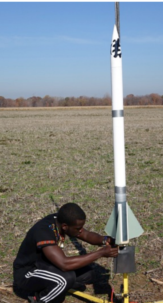
Kofi Bosompin (left) made three attempts to fly a cluster of 3-AT Economax G76 motors but only got one motor to ignite each time as can be seen in the photo (right)
