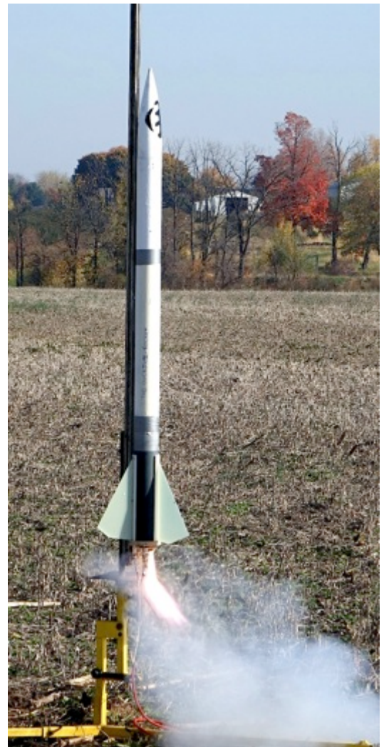
Kofi Bosompin (left) made three attempts to fly a cluster of 3-AT Economax G76 motors but only got one motor to ignite each time as can be seen in the photo (right)
