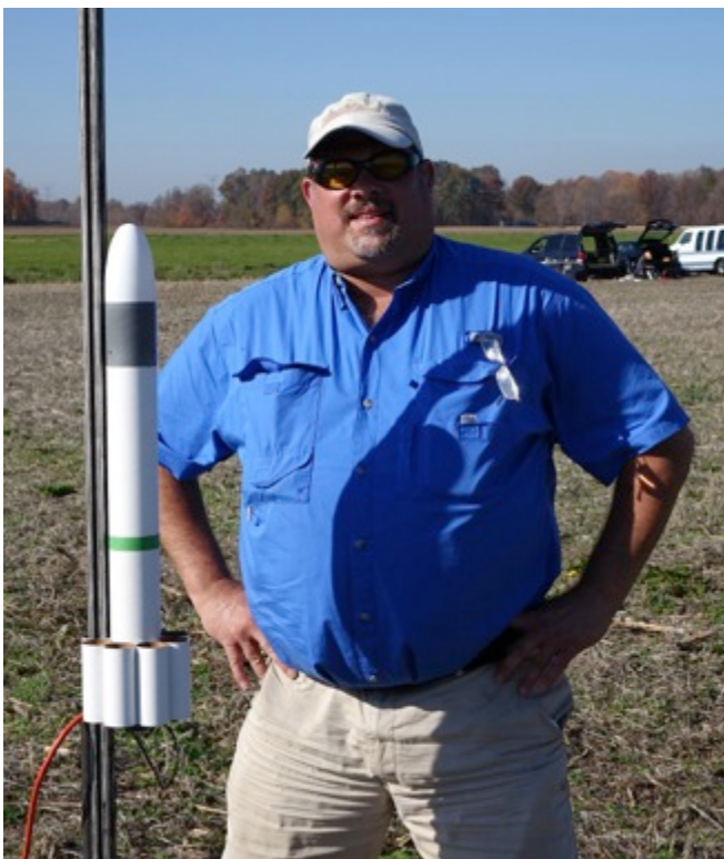
John Ulizzi (left) poses with his SM-80 tube/ fiin rocket prototype, which he flew many times that day. Shown at right is the first flight on a D12. He also flew it on an E12 to 355 feet, an E30 to 550 feet and a F26 to 31 feet.
