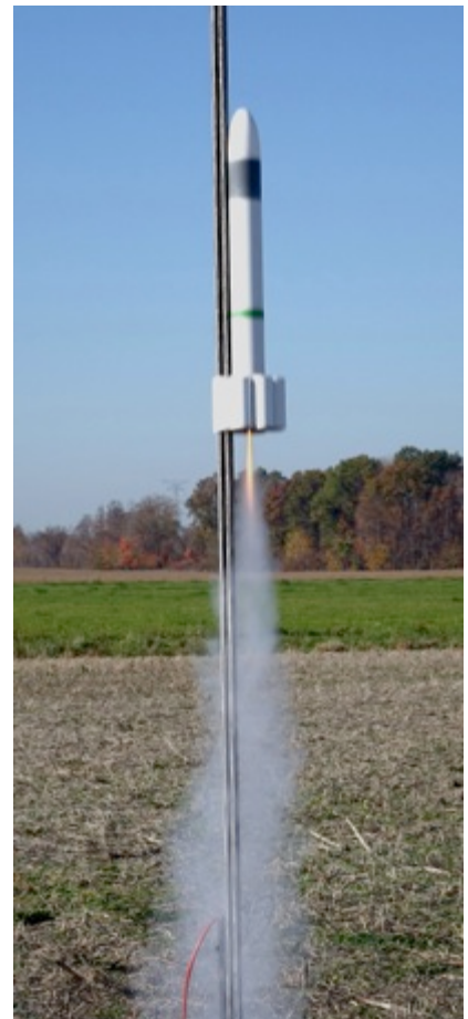
John Ulizzi (left) poses with his SM-80 tube/ fiin rocket prototype, which he flew many times that day. Shown at right is the first flight on a D12. He also flew it on an E12 to 355 feet, an E30 to 550 feet and a F26 to 31 feet.
