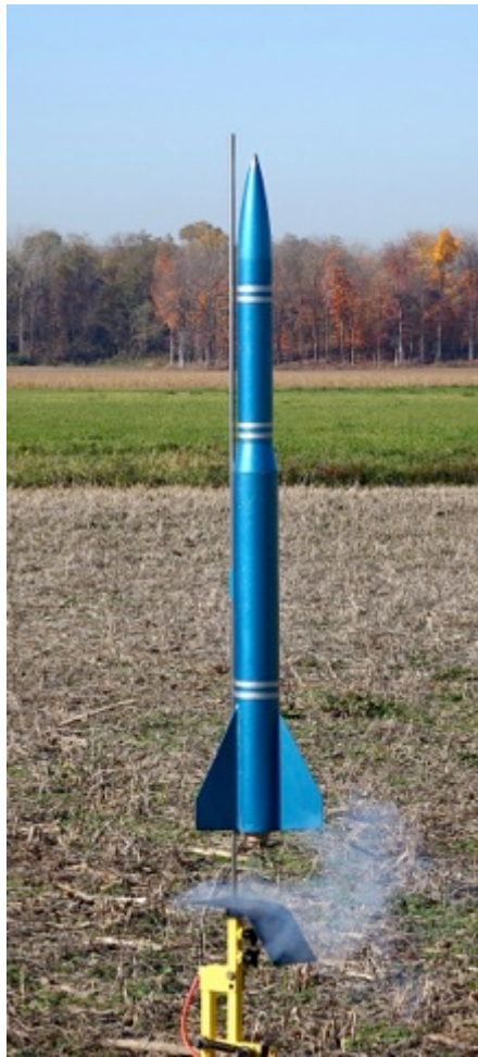
Steve Eves (left) flew his LOC/Precision "Expeditor" on a Research Red I159 motor (center). The second flight of Mark Coburn's "Expeditor" (right) on a J460T motor, which took it to 3700 feet.
