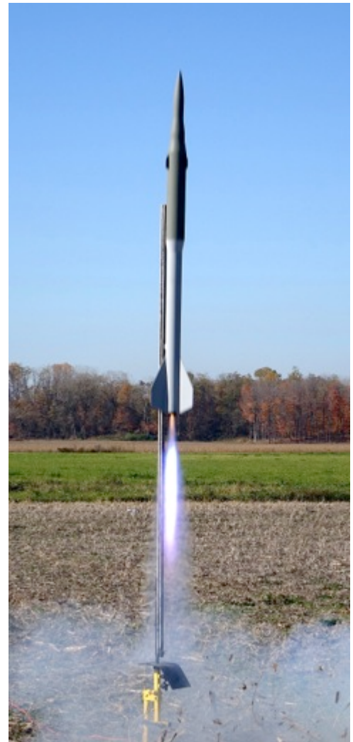
Pat Ralph (left) with his scratch-built "Probe" on its maiden flight (in primer gray) on a CTI I303 Blue Streak to 2948 feet (right).
