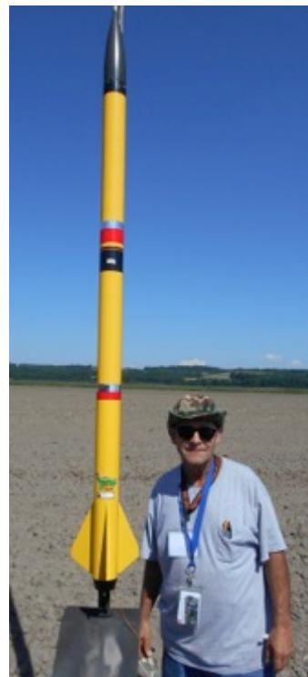
Mark Coburn flew his extended LOC EZI-65 (above left) with a Research J340 using NASSA K2 Fast propellant to an altitude of 2500'. He later flew his LOC I-Roc (above center) with an AT J570 to an altitude of 2200'. He flew his 3" HyperLOC (above right) with an AT I284 to an altitude of 3420'. He also flew his LOC Magnum with a Research K350 motor using NASSA K2 Slow propellant, which flew to 2200'. Mark calls all his rockets "Bug Juice" as the decal on his rockets shows.
