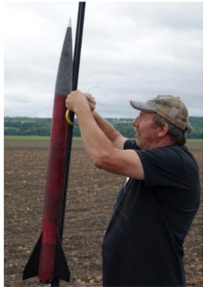
Steve (left) turns on the altimeter on his Wildman "8-Ball" which he flew with a 38mm I250 Research motor using NASSA K2 Fast propellant.
