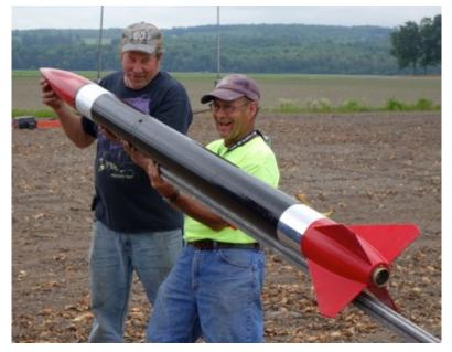
Steve and Mark (left) load Steve LOC/Precision "Syonic" onto the pad. This is one of the original rockets that Ron Schultz built for his catalog shoot back in the 80's. It flew on a Research J480 using NASSA K2 Fast propellant to 2555 feet and had a perfect recovery.
